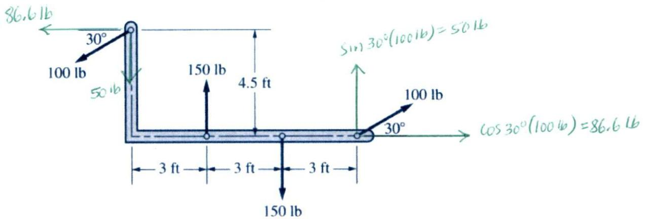
$$\begin{aligned} M_f &= 86.6 \text{ lb}(4.5 \text{ ft}) + 50 \text{ lb}(9 \text{ ft}) - 150 \text{ lb}(3 \text{ ft}) \\ &= 389.7 \text{ lb}\cdot\text{ft} + 450 \text{ lb}\cdot\text{ft} - 450 \text{ lb}\cdot\text{ft} \\ &= 390 \text{ lb}\cdot\text{ft} \curvearrowright \end{aligned}$$
